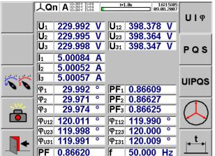
Further sub-menus provide access to power measurement (PQS), vector diagram, phase-phase voltage U, phase angles U-U, I-I are directly accessed via the soft keys. Ranges can be fixed, results can be stored in internal memory. The exit key is used to return to the next higher menu level.
