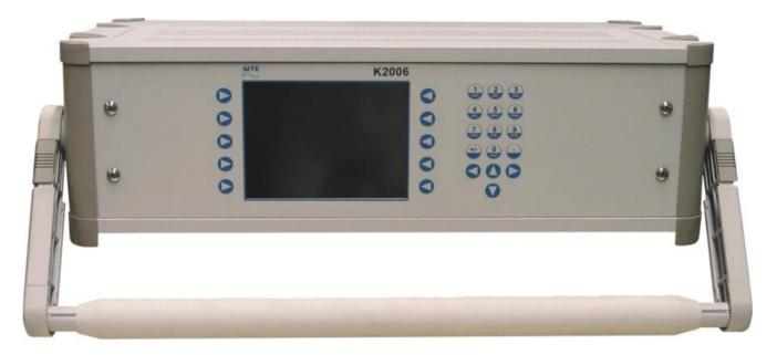
The K 2006 is a three phase comparator which has been especially developed for universal laboratory and test area use. It is intended for checking and calibration of reference standard power and energy meters, for calibration of precision current and voltage sources and for verification of electrical standard measurements and electricity meter test systems.
