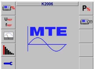
The main functions, error %, test against U-ref, f-ref, load values UI<sub>0</sub>, harmonics and basic system settings are directly accessed with soft keys.
